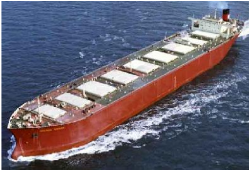
Fig.18 Freighter Ship MV Orenda Bridge (70000+ Tons) with Doxford 76J8 20000 HP - OPE
