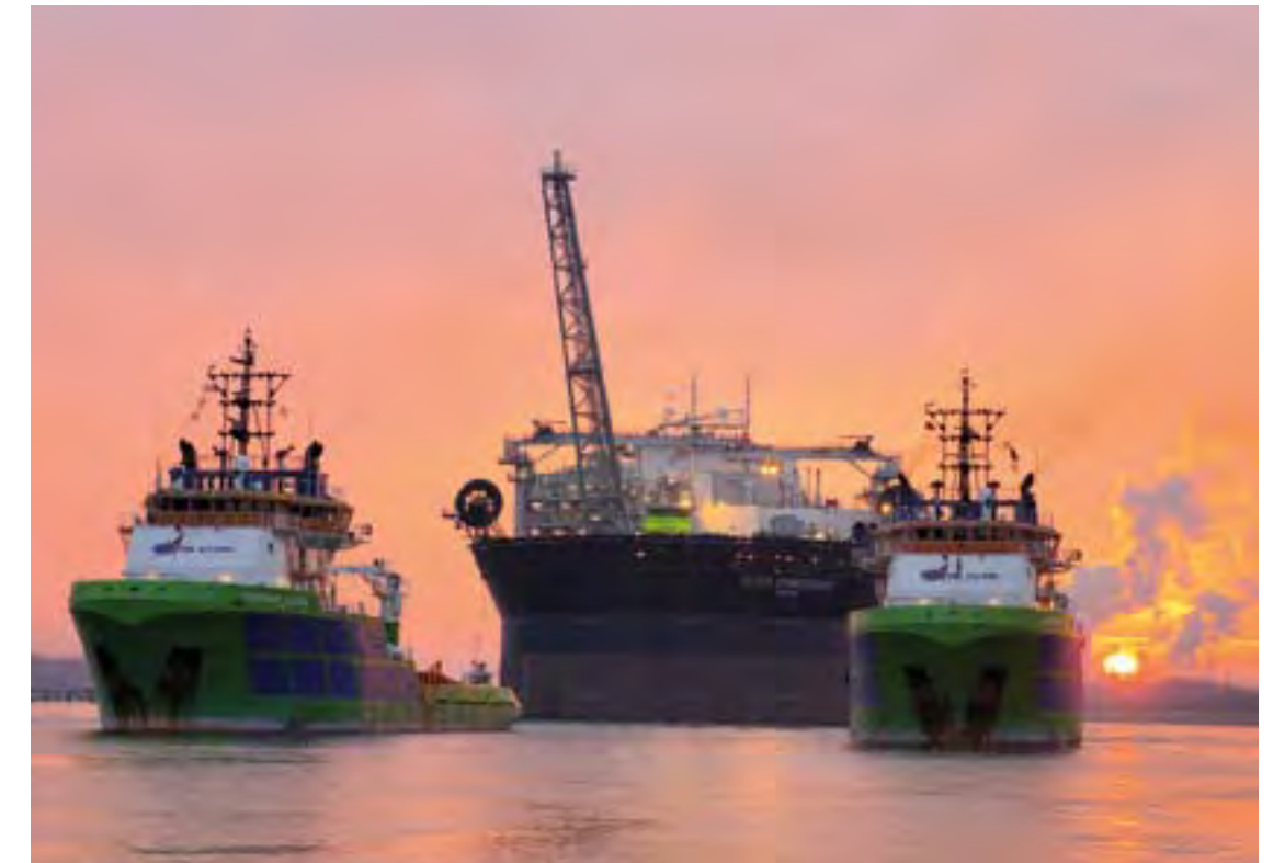
TOP FPSO Piranema Spirit , the first cylindrical FPSO, is operating for Petrobras on the deepwater Piranema field off Brazil. Installed to operate at a depth of 1,100-metres, she is currently interconnected to seven wells, some for extraction of oil and some to re-inject water into the seabed. Teekay Collection ABOVE In August 2008 FPSO Hummingbird Spirit (then named Sevan Hummingbird ) became the first cylindrical FPSO to be installed in the North Sea. Her ability to receive helicopters even during severe winter storms and the fact that she experiences no processing restrictions in relation to weather conditions, have demonstrated the suitability of the Sevan design for operations in harsh environments. Teekay Collection
