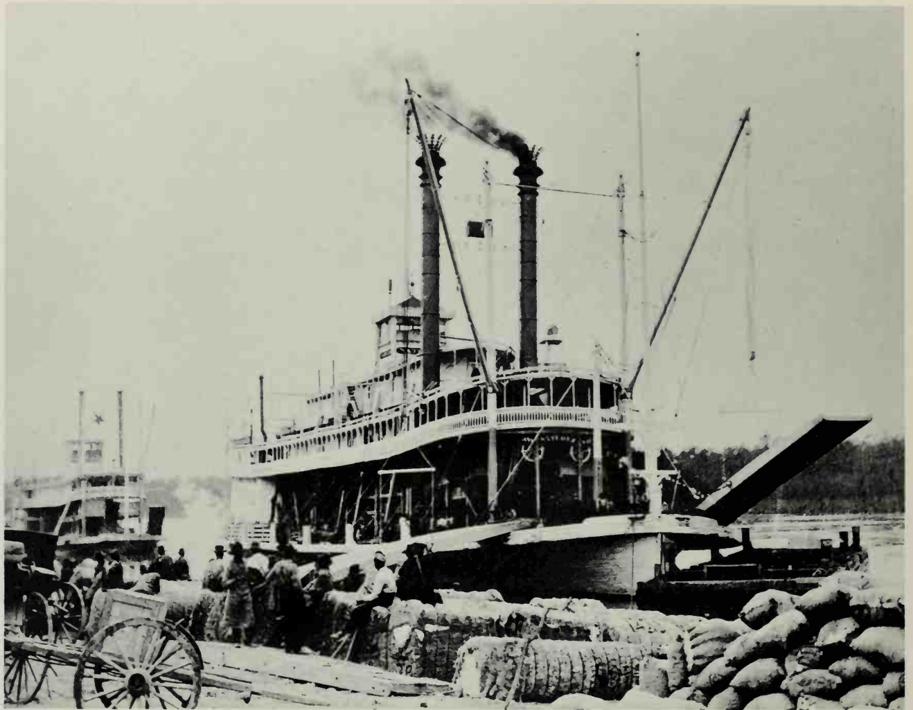
268. The Natchez (the eighth of the name), built in 1891. She was a sternwheeler 225 feet long, forty feet wide, and six feet deep in the hold.
