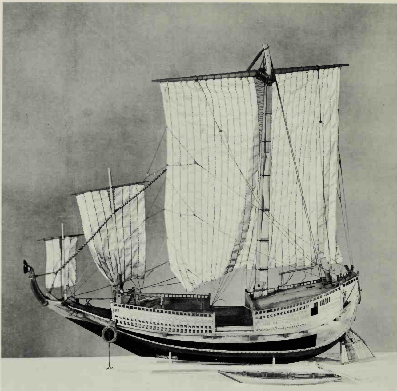
200. Modern model of a large (106' \times 34' \times 10') Japanese coaster of the early nineteenth century. The tall square sail somewhat resembles those of ancient Egypt (compare illustration 17) and, like them, was probably effective only with a following wind.
