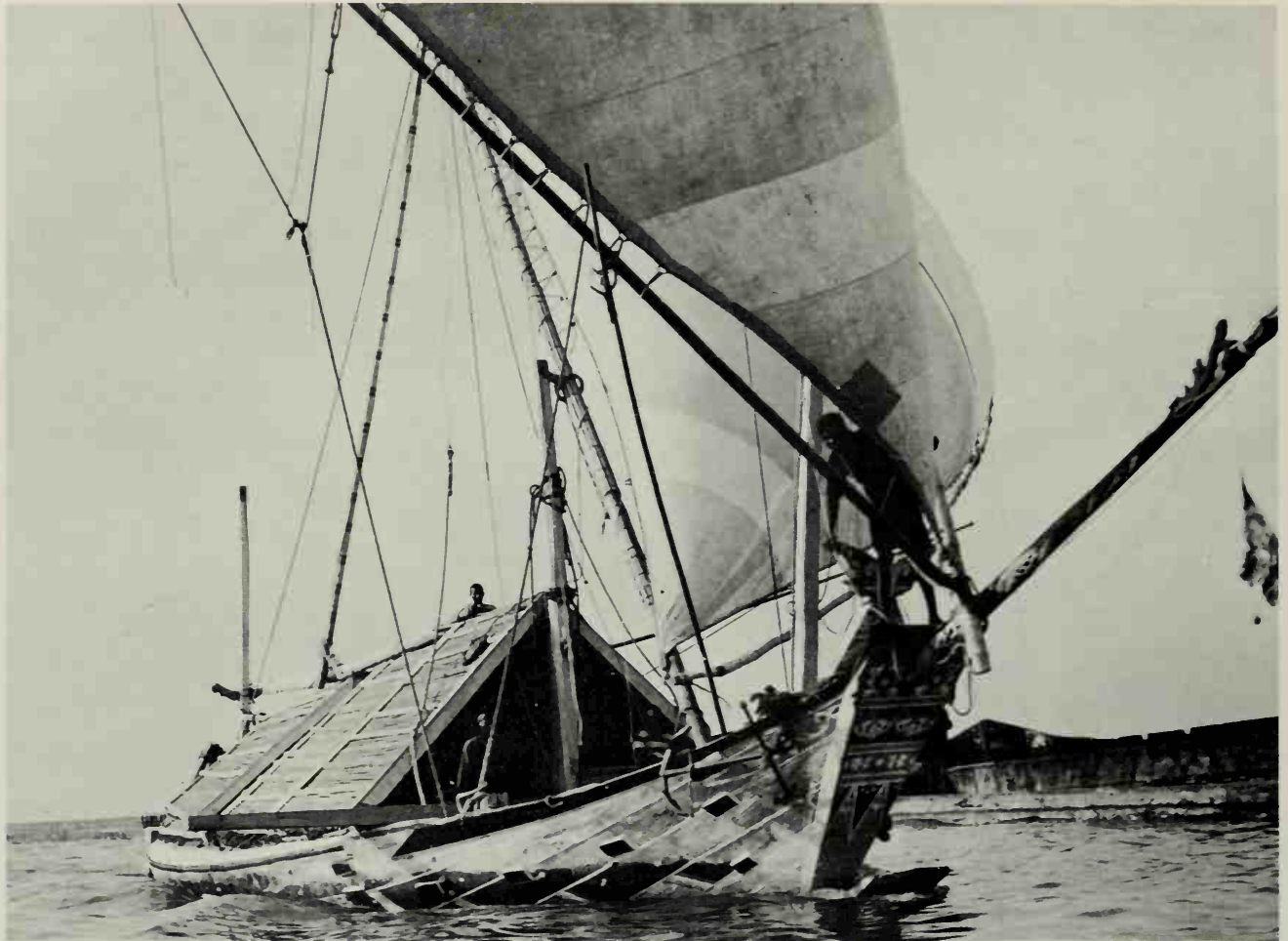
248. A Javanese prau under sail. The bamboo pole standing behind the cabin reaches up to the main yard and serves as a prop for it.
