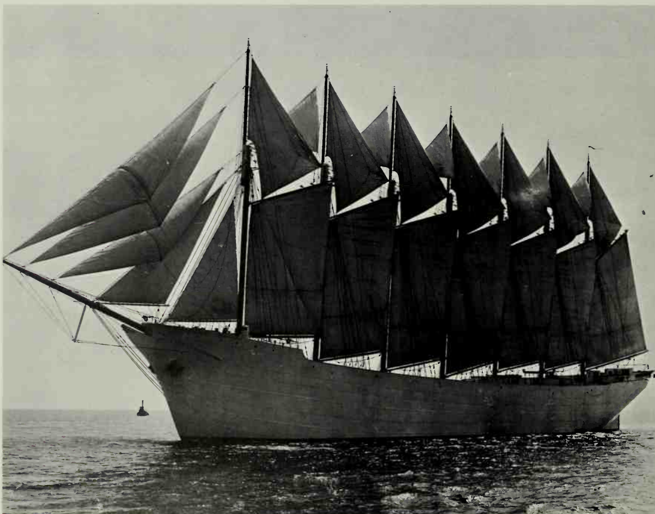
183. The seven-masted, steel-hulled Thomas W. Lawson . She was 395' long, 50' wide, 35.2' deep in the hold, and 5218 tons. Her schooner rig and various mechanical aids enabled her to do with a crew of only sixteen men.
