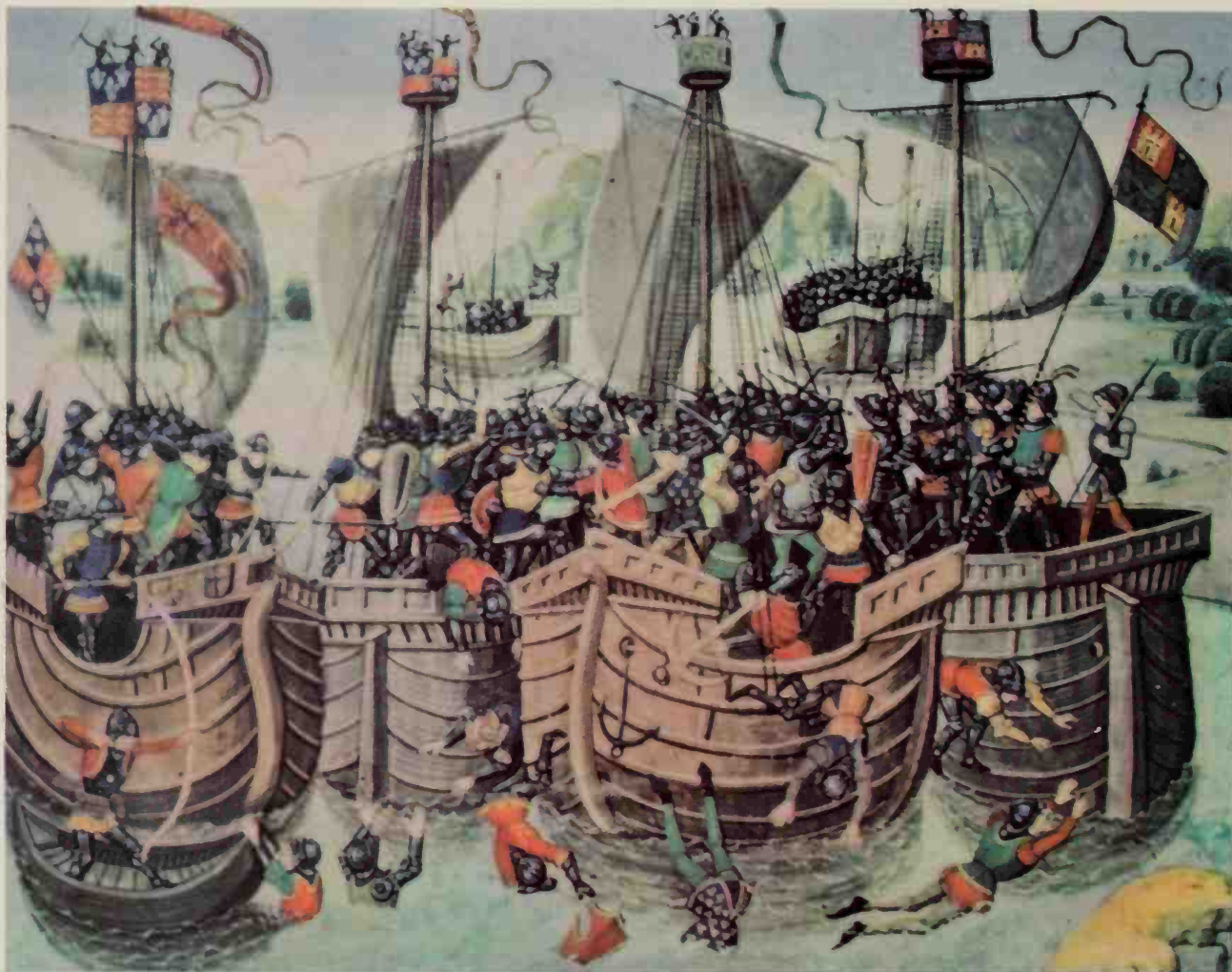
85. Fifteenth-century cogs in action. These are examples of the cog in its prime, a stubby but massive and sturdy ship with a mast strong enough to support as many as four persons in its top. The sails carry reefpoints.
