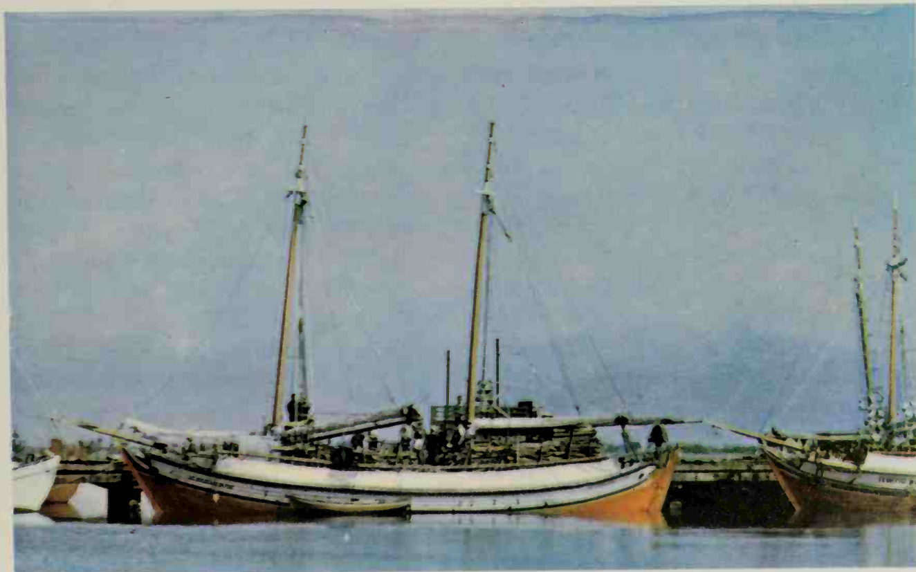
231. A modern large Greek caïque. The shape of the hull is typical: sharp stern with outboard rudder, low waist raised by canvas strakes, raking prow. The sails are balance lugs, but nowadays are not often raised; skip-pers prefer to use their diesel motors. See page 198.
