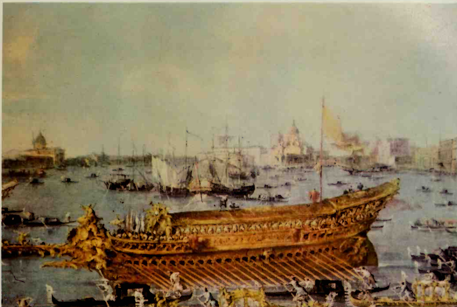
143. The Bucentaur , the monumental state barge of Venice's doges, in its eighteenth-century form. In weight and structure and general shape, the Bucentaur was a galeass; instead of fighting castles and other accoutrements of war, it carried spacious quarters and gorgeous decoration. This particular version was 114 feet long and twenty-four feet wide, and had twenty-one sweeps a side each thirty feet long and manned by four or five men.
