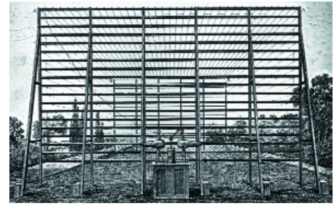
Francis Ronalds’ eight miles of wire set up on his lawn for experiments on the velocity of electricity.
