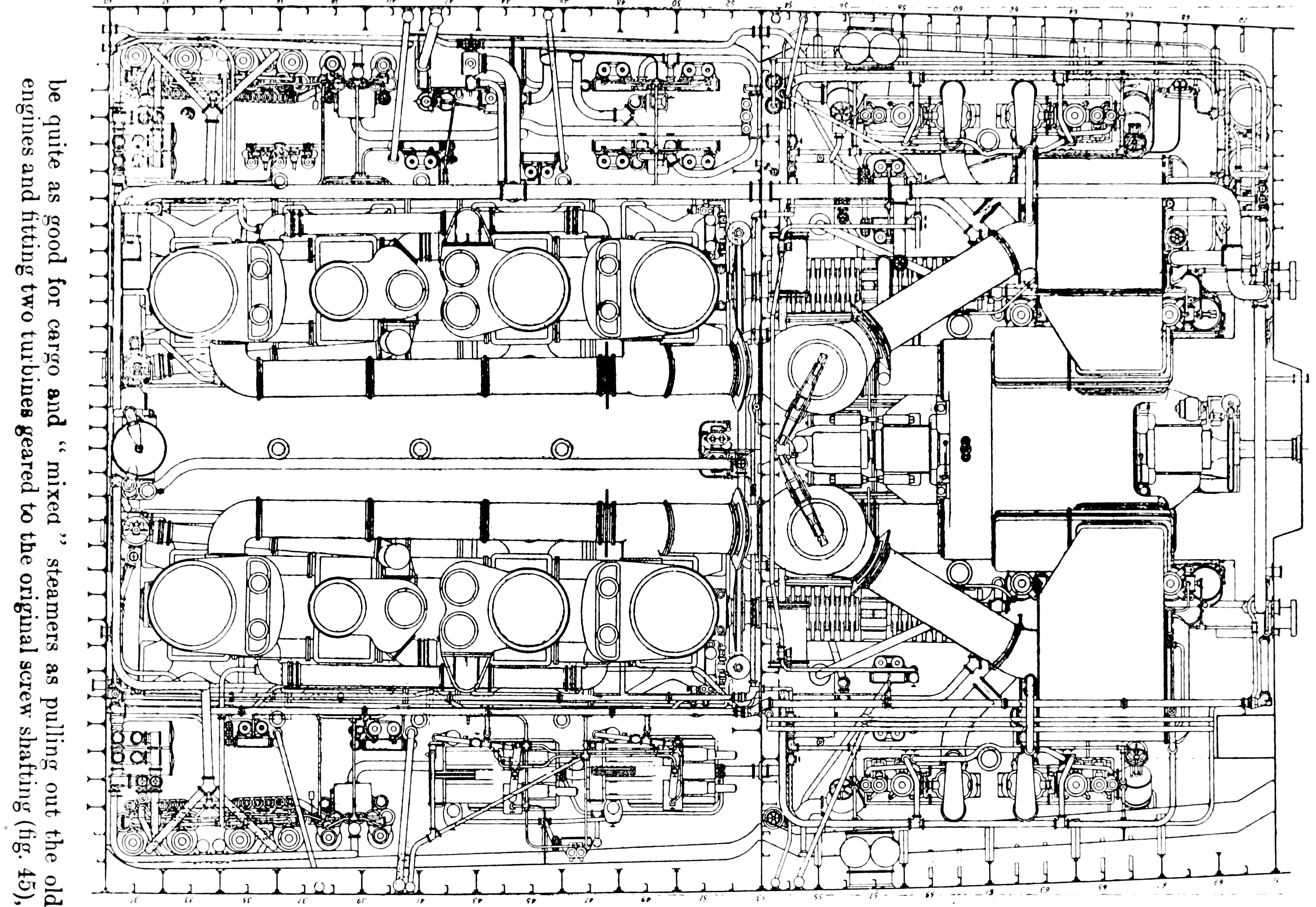
Fig. 44.—Plan of Engine-Room of R.M.S. "Olympic," 50,000 tons displacement. Two Triple-Expansion Reciprocators and One L.P. Turbine, 55,000 H.P.
