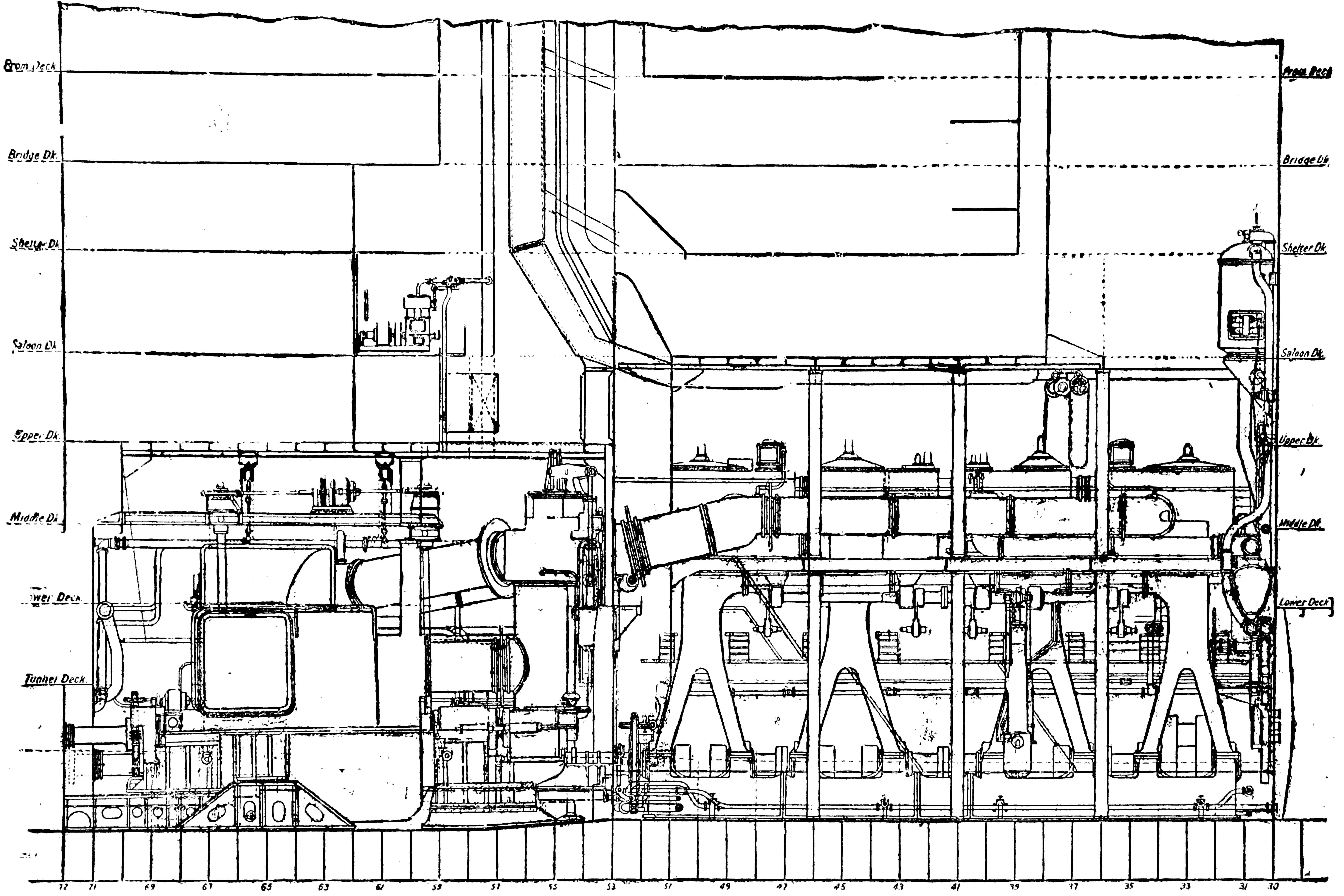
Fig. 43.—Longitudinal Section through Engine-Room of R.M.S. "Olympic," built by Harland & Wolff, Belfast.
