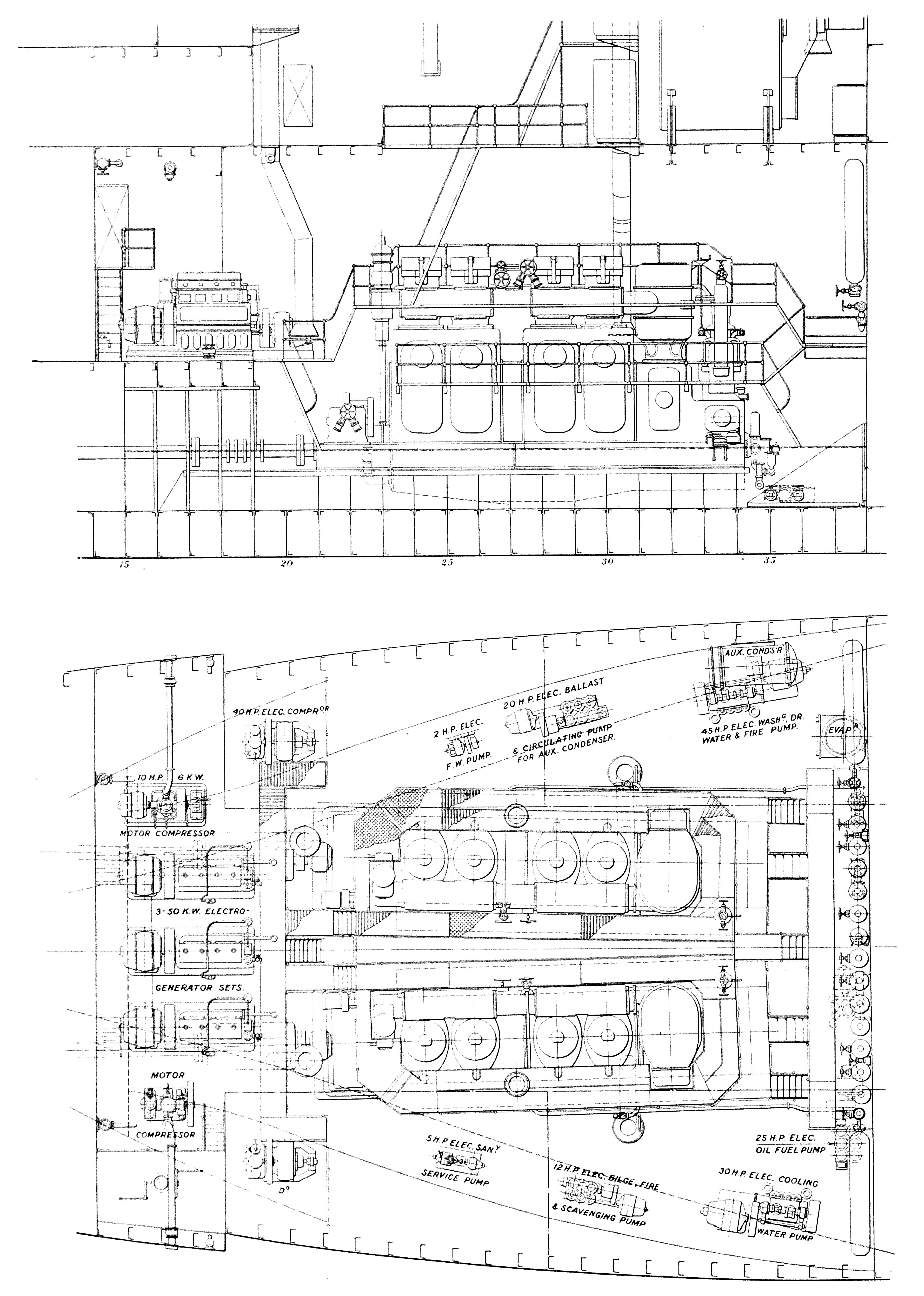
The Motor Tank Ship "Capena." Elevation and Plan of Machinery Space.
