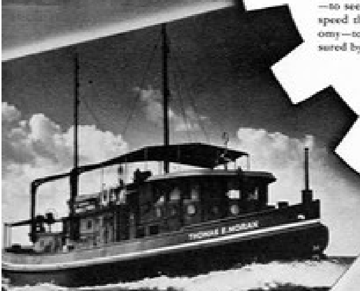
THE THOMAS E. MORAN , one of the two new all-diesel tugboats of the Moran Towing and Transportation Co., Inc., America's largest towing concern. Both boats are GM Diesel-powered for Diesel Electric propulsion and auxiliary service.
