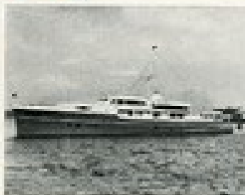
SAVITAR , 118-foot, all steel, DeLor Cruise-master, one of six palatial yachts, each powered with two GM Tandem Twins.
